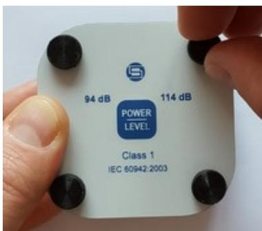
f) holding the cover with one hand fasten the fixing screws
