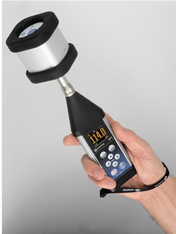
Picture 2. Calibration of the SVAN 971 sound level meter with a 1/2" measurement microphone
