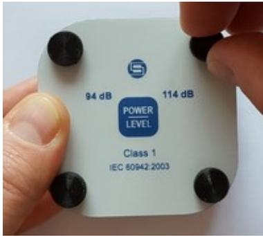
b) holding the cover unscrew four fixing screws with your fingers
