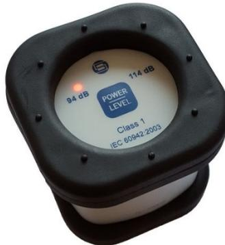
Picture 4. The top view of the SV 36 calibrator with one diode on
