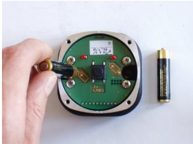
d) put new batteries in place of the discharged ones with polarization as indicated on the printed board and calibrator's case
